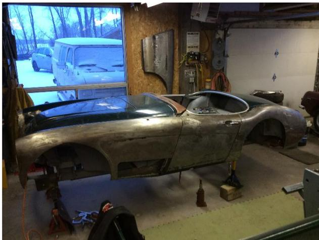
After two years of disassembly, reassembly x 100, replacement of sills, two outriggers, shut-face pillars and inner wing dog legs, boot floor, and much fabricating of sheet metal parts, the car is as you see it now. The doors open and close, are in line with wings, have lock and striker plates in, and have the all-so-important correct distance from the sills. I could go on like a car guy, but I won't, or will I?
