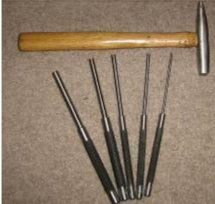
The tools needed are few and easily obtainable. Shown here are the punches in a variety of sizes suitable for these repairs along with a light hammer. Another tool that is nice to have, but not absolutely necessary, is a metal file. You will also need sandpaper from 120 grit all the way to 1000 grit for final sanding, depending how smooth you will want your finished piece to look like.
