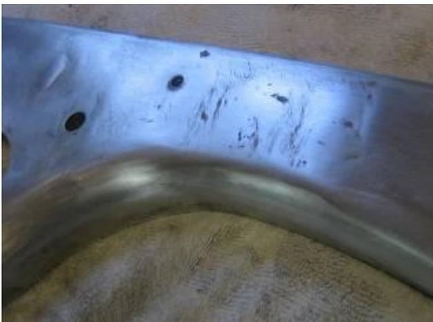
This photo shows the same general area again, this time one can see the scratched areas surrounding where repairs will be done. These scratches were done by using a metal file and it easily highlights the high spots in the metal surface.
