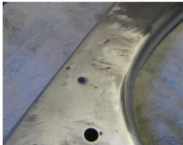
Here is a close-up of the largest corrosion spot, just above the screw hole used to secure the dashboard to the chassis. For the purpose of this demonstration, this is the corrosion spot I will concentrate on.
