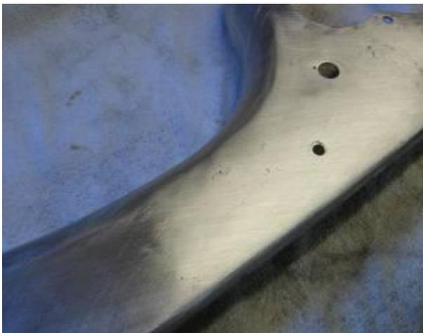
This last photo shows the finished product, in this case done only to 400 grit. Later on, before being primed, I would sand it with 600 paper, then finish with wet sanding to 1000 grit.
