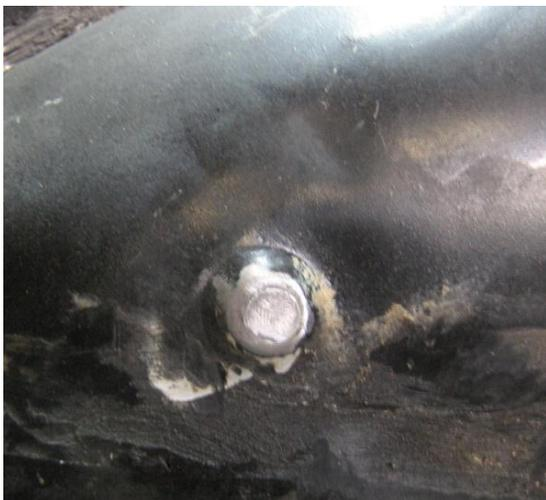
Step #3 is to weld the sheet metal in place and then clean your weld. For that purpose I use an air angle die grinder with the 50 grit 3M sanding disc until I get a smooth surface.
