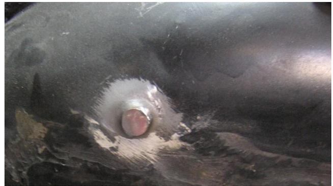
Illustration #4 shows the surface after the sanding is completed.
