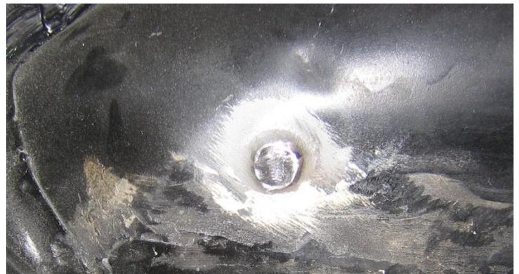
All there is left to do now is to locate the centre spot of your newly repaired surface and drill the new hole to the size appropriate to the item going through it, in this case a 3/8" hole for the flat head, countersunk machined screw used to secure the side support for the folding backrest.
